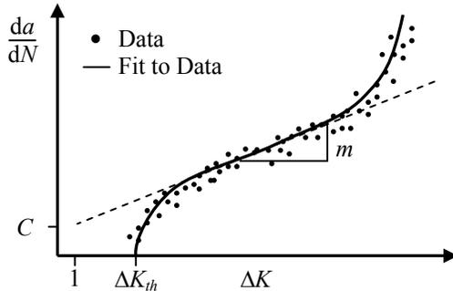
Figure 1. Crack growth data and Paris model fit.
