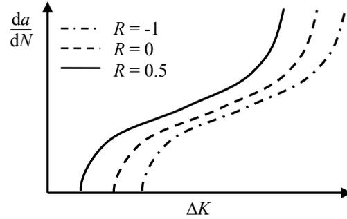
Figure 2. Fatigue crack growth curves for different stress ratios  $R$  for constant amplitude loading.
