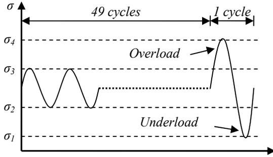
Figure 5. Repeating block loading used for simple variable amplitude fatigue predictions.
