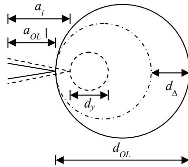
Figure 4. The current, overload, and underload crack geometries and plastic zones used in  $M_p$ .
